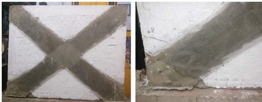
Fig. 13. Crack pattern for CLY-S-GFRP-X with rocking at connection.
