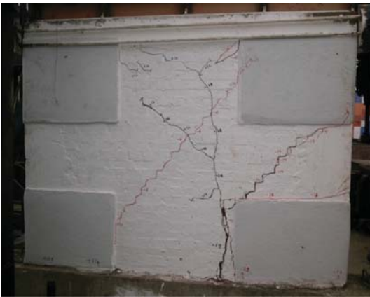
Fig. 11. Crack pattern for CLY-S-FERRO-C.
