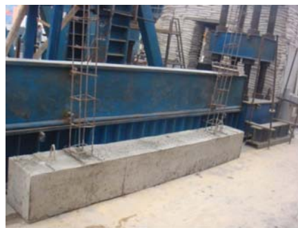
(a) Footing with column reinforcement
