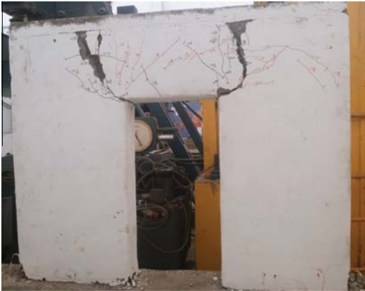
Fig. 19. Crack pattern for CLY-D-FERRO.
